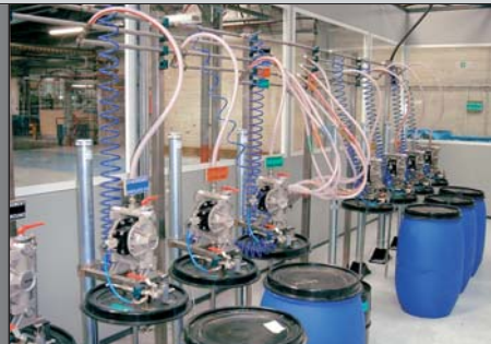
1/2" diaphragm pumps installed in a colouring process
